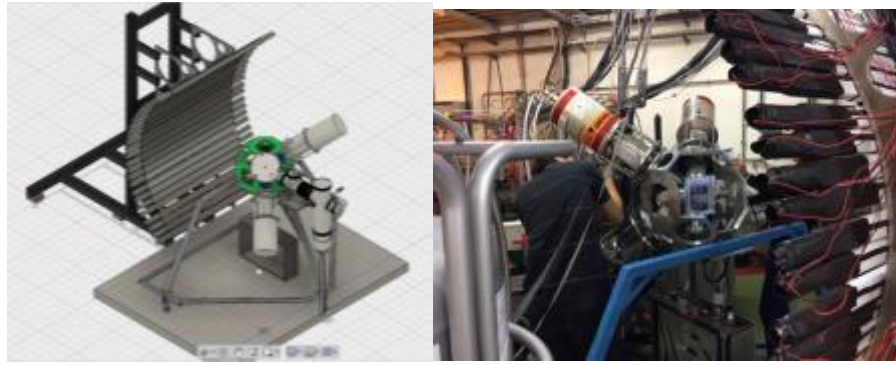
Figure 4: (left) Schematic drawing of the IDS setup using four clovers combined with the IDSND detector and support at 1 m flight path. (right) picture of IDSND commissioning run for ISOLDE experiment IS609.
