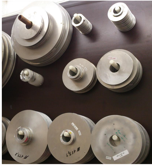
Figure 5.3: Different size aluminium reels for fiber sample spooling
