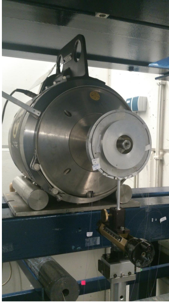
Figure 5.2: The Gammamat TK1000 ^{60}\text{Co} irradiation system with reels mounted on it
