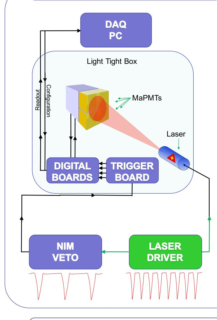
A pulsed laser with 405 nm wavelength was aligned with the centre of the EC, inside a light-tight box. The pulse rate was varied up to 20 MHz at the external laser driver.
