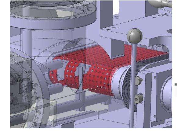
Beam instrumentation RF shielding
