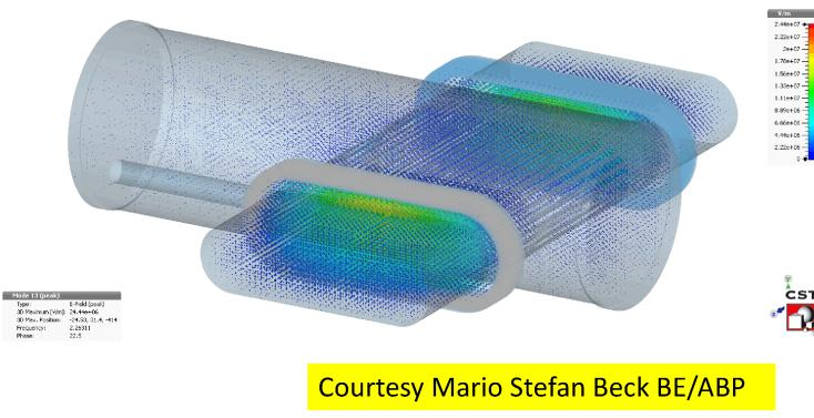
Results of a bellow resonance frequency analysis used to design the bellow and shielding
