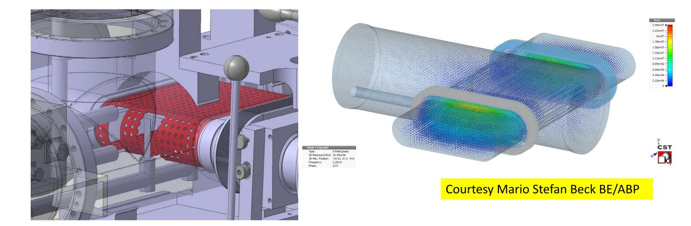
Beam instrumentation RF shielding Results of a bellow resonance frequency analysis used to design the bellow and shielding
