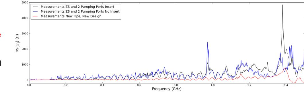
Beam impedance measurement using wire installed on a spare ZS with simplified elliptical beam pipes (both ends)
