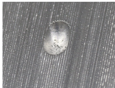
Figure 4.16: Pin insert in the winding wheel. It has steep edges parallel to the fibres to ensure a good alignment.
