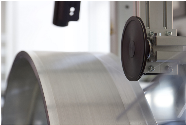
Figure 5.16: One-sided mounting of the positioning spool of the serial winding machine. The fibre is guided with the lower part of the spool which enables a large spool and a short distance to the winding wheel.
