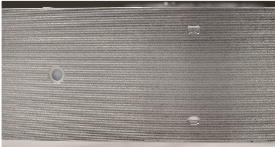
Figure 5.9: Different shaped prototype pin holes in the small Dortmund wheel. The cylindrical hole on the left is realised with a Teflon ® inlet to avoid the need of a release agent.
