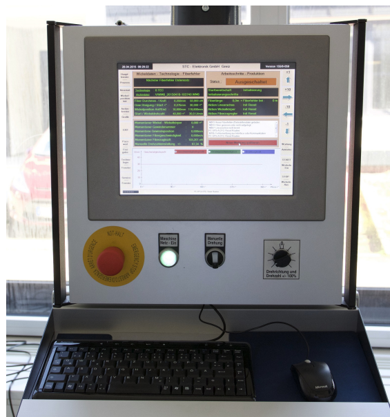
Figure 5.17: Control PC of the serial winding machine. The interface is a mixture of hardware knobs/switches and touchscreen software control.
