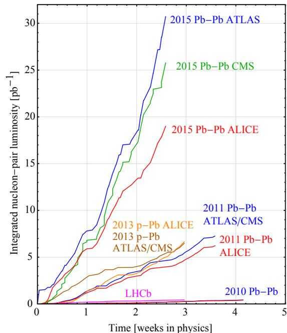
Figure 6: Nucleon-nucleon integrated luminosity in each experiment in all LHC heavy-ion runs to date [1, 12, 13], from the first declaration of Stable Beams.
