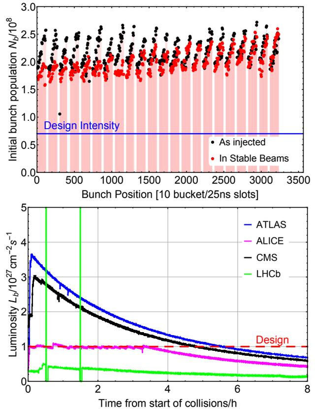
Figure 5: Bunch populations at injection and start of collisions (top) and luminosity evolution (bottom) in fill 4720 (the LHCb luminosity contains two unphysical glitches).
