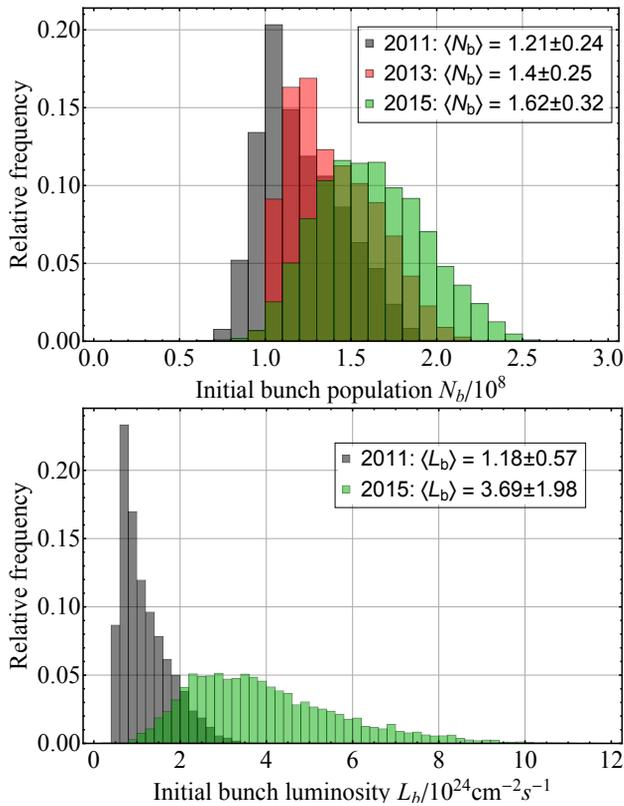
Figure 4: Top: Distribution of bunch populations at the start of collisions over all Pb-Pb fills in 2011 and 2015 and all p-Pb fills in 2013. Bottom: Distribution of initial bunch pair luminosities over all Pb-Pb fills in 2011 and 2015.
