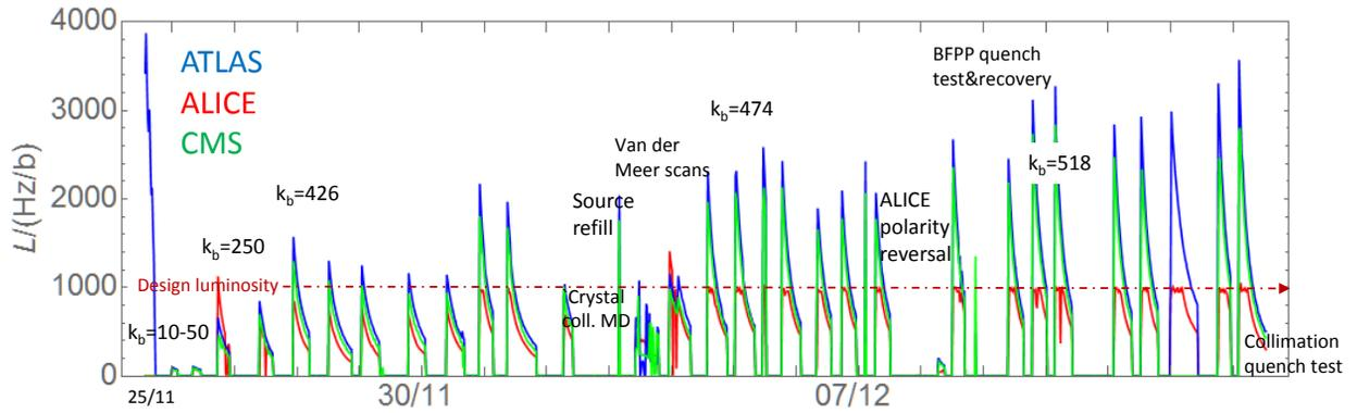
Figure 3: Luminosity for 3 of the 4 experiments, during the 2015 Pb-Pb run showing the progressive increase of stored bunch number  $k_b$  and the various interruptions of regular data-taking. The dashed line shows the design luminosity [3].
