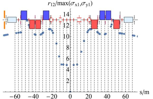
Figure 2: Beam-beam separation in units of the larger horizontal/vertical beam size close to ALICE. Vertical lines represent possible encounter points.
