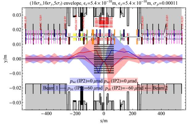
Figure 1: Vertical beam envelopes around the ALICE experiment in physics conditions with spectrometer bump angle  $-77 \mu\text{rad}$ , external bump  $+137 \mu\text{rad}$  for Beam 1.
