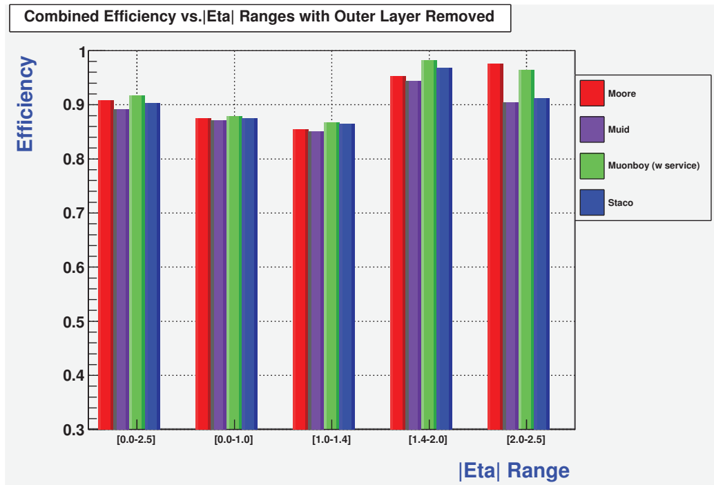
Figure A.13. Reconstruction efficiency for muon spectrometer and combined algorithms, under the removal of the outer chamber-layer of MDTs, for various pseudo-rapidity ranges.
