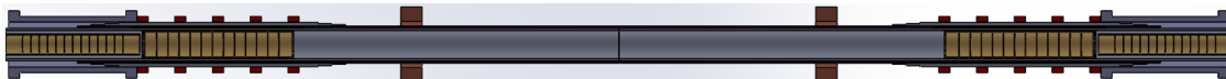
Figure 8. Schematic of the internal portion of the ALPHA-g device, rotated to the horizontal plane. A complete antihydrogen synthesis and trapping region (Penning trap and atom trap) occupies each end (top and bottom) of the machine. The central analysis region confines antiatoms using copper mirror coils and a reduced-strength octupole.
