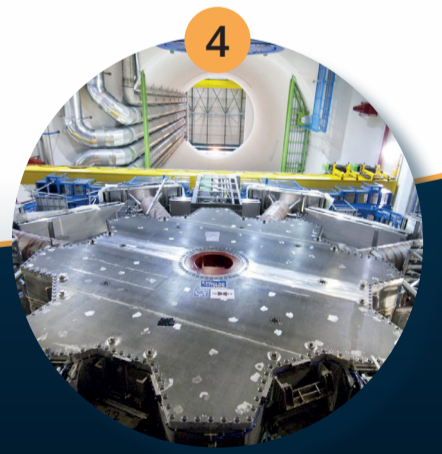
Magnet System bends the trajectories of each charged particle to allow the measurement of its momentum
