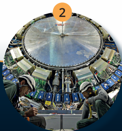
Calorimeter measures energies carried by neutral and charged particles
