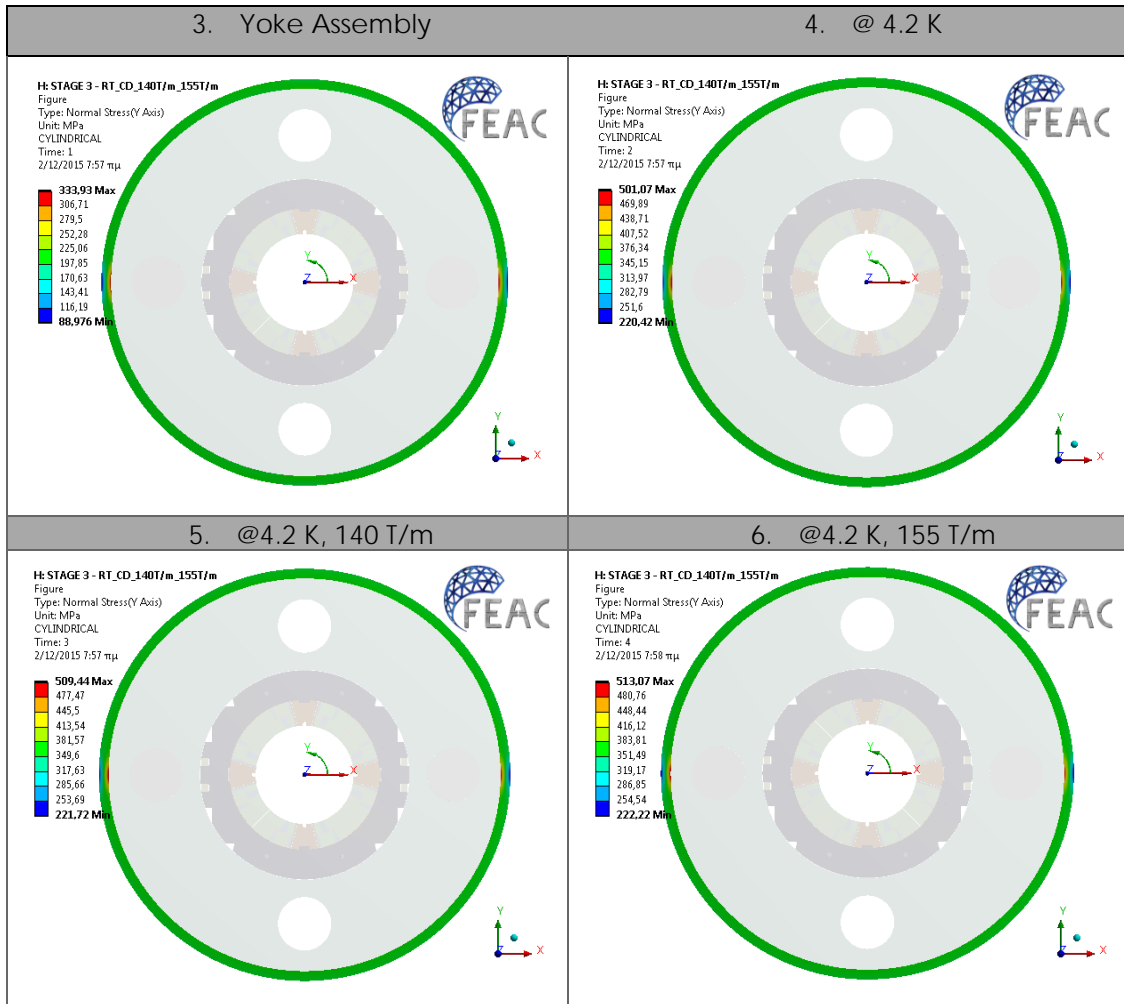
Figure 37: Azimuthal stress [MPa] at all stages
