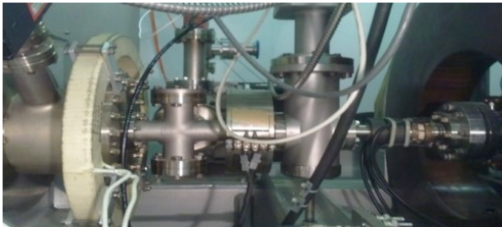
Figure 1.6: The effect of first focussing coil (in the middle of the picture) has to be compensated near the cathode by the bucking coil (on the left). On the right, the first of the 14 Helmholtz coils is visible.
