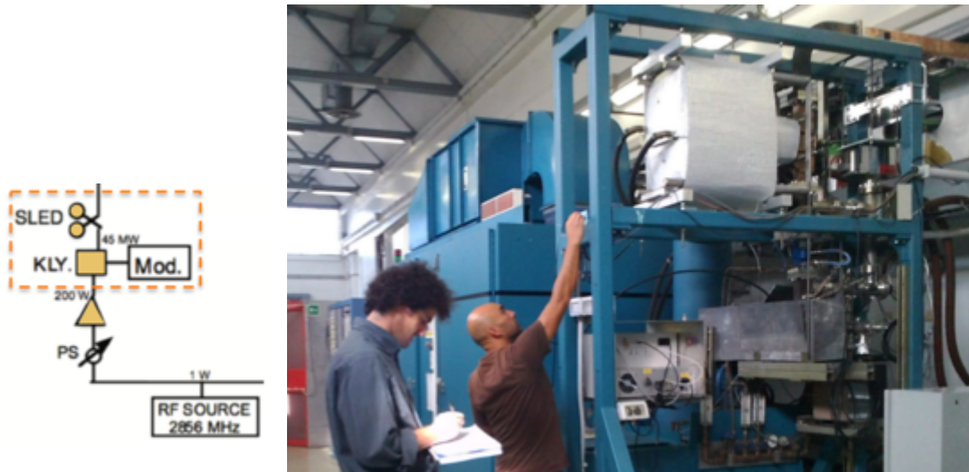
Figure 3.1: The RF power station (left, logical scheme; right, photograph): the 1 W RF from the 2856 MHz source, pre-amplified to 200 W by the RF driver, is amplified up to the maximum power by the klystron, fed by the modulator, and compressed by the SLED, prior to be distributed by the waveguide network to the accelerating sections.
