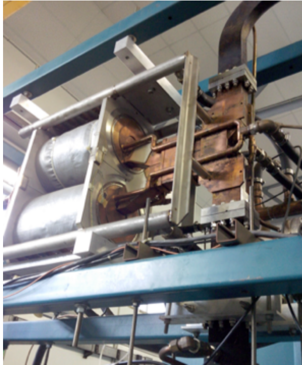
Figure 3.6: The SLED device is composed by two (cylindrical) resonant cavities, connected by a 3 dB hybrid coupler, taking as input the power from the klystron (just below, not shown in the picture) and output to the waveguide network towards the accelerating sections.
