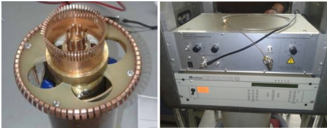
Figure 1.3: Electron gun cathode socket (left), and isolated high voltage station with new pulsing system (right).
