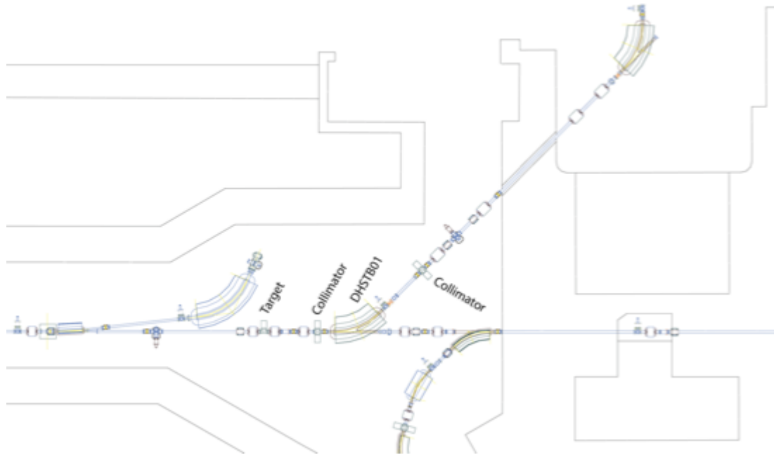
Figure 1.10: Layout of the original BTF beam attenuation and extraction system (until 2004) with the main elements (target, dipole, collimator) on the main injection line.
