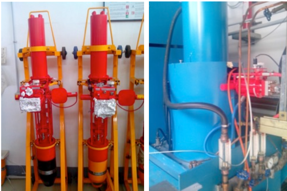
Figure 3.5: Left: two klystrons Thales TH2128C (exhausted); right: the klystron installed inside the cooling oil tank and surrounded by its focalizers.
