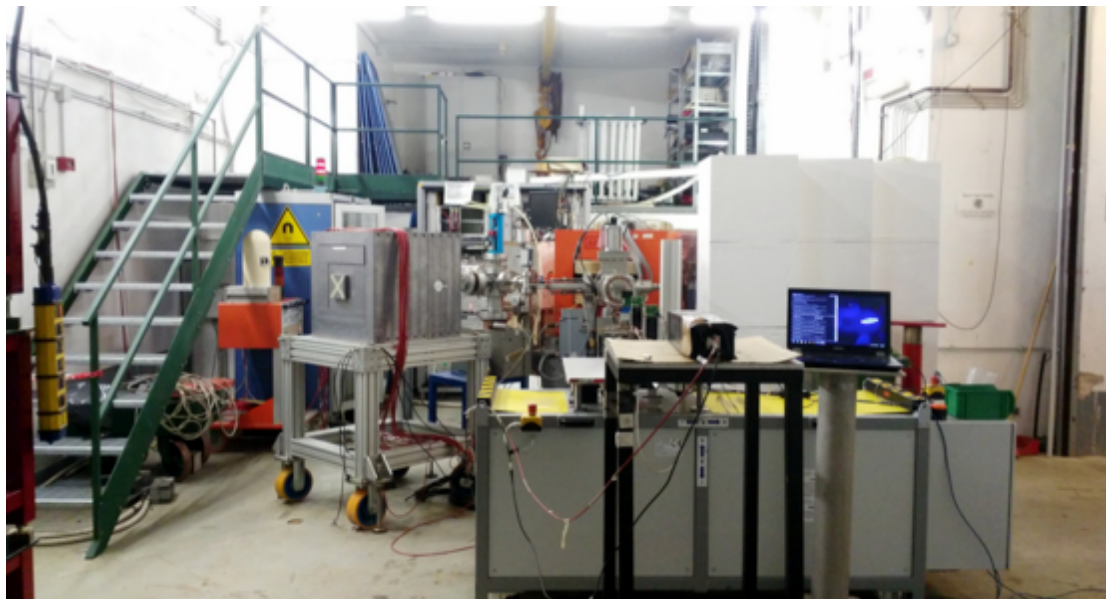
Figure 3.17: Picture of the present BTF beam-line and experimental, showing the useful user area at the exit of the DHSTB02 45° dipole (orange), equipped with diagnostics and remotely controlled trolley. The lead/polyethylene cubic shielding of the neutron production target is also visible at the exit of the straight beam pipe (on the left).
