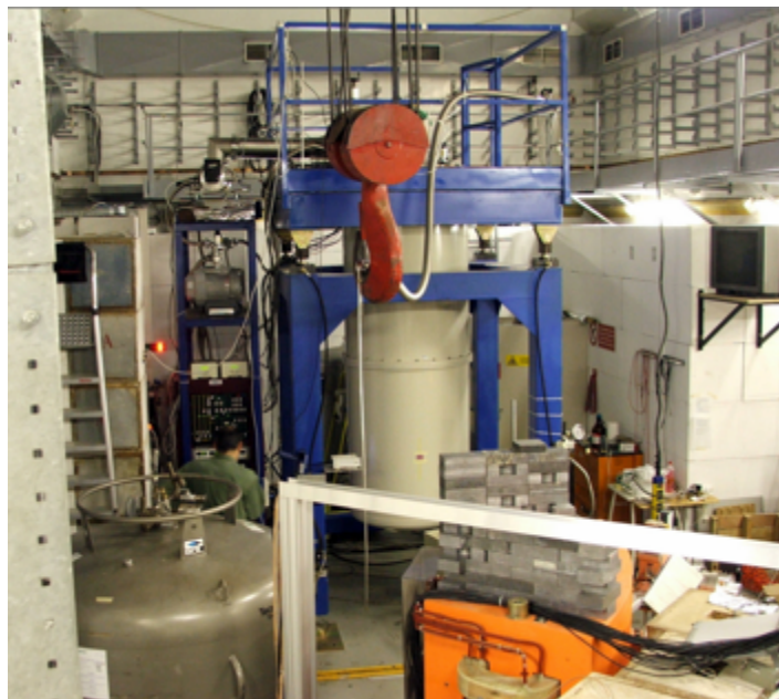
Figure 1.28: The RAP experiment took data at BTF with high intensity 510 MeV electrons from 2003 to 2007, measuring the effect of thermo-acoustic expansion on a super-conducting resonant antenna (inside the large dilution cryostat), made by an Aluminum cylinder, 1:6 of the NAUTILUS gravitation antenna.
