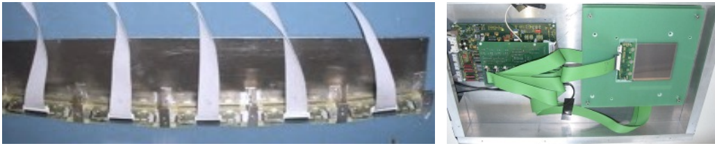
Figure 2.2: Silicon micro-strip tagging modules (left), placed along the curve beam-pipe, and active Silicon micro-strip target (right).
