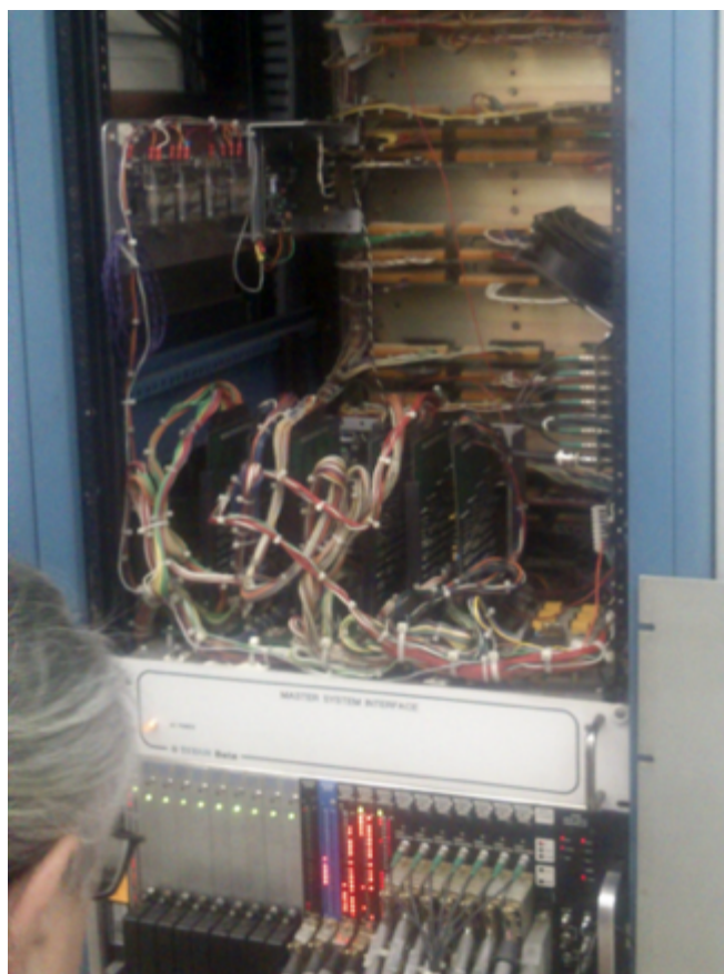
Figure 3.8: Interlock analog signals routed to the control custom-built board. All signals are readout by a CAMAC-bus system (visible at the bottom of the picture).
