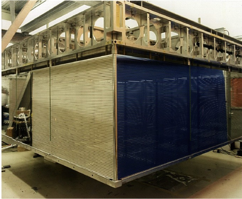
Figure 15: The outside view on one of the Vertex TPCs. Mylar strips are visible surrounding each side of the cage.
