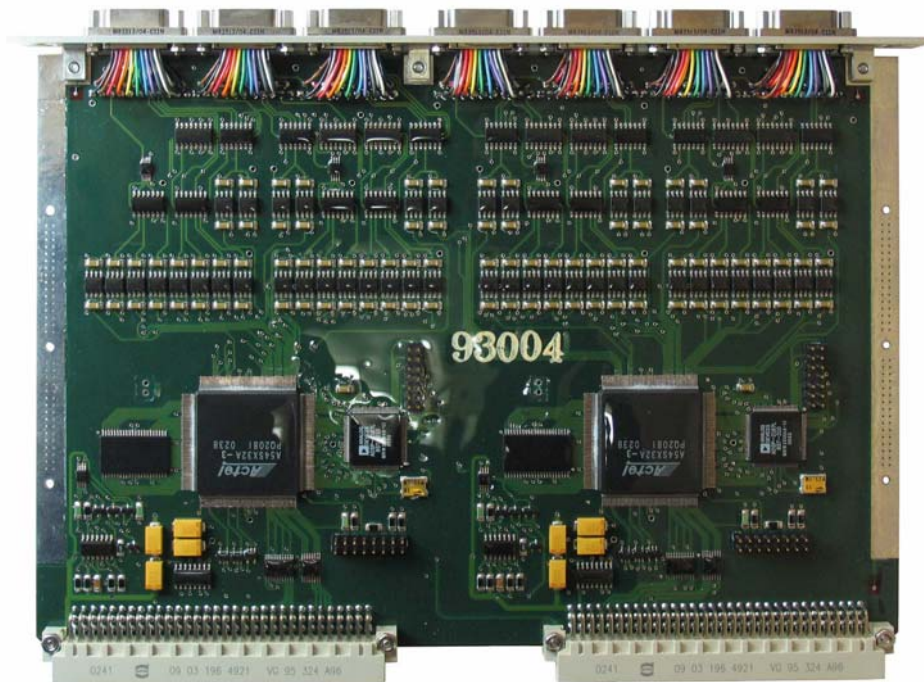
Figure 2.13: UDR2: U Data Reduction, version 2. The different parts of the UDR2 can be clearly distinguished: The two redundant CDPs and the detector specific part, which is located close to the connectors for the front-ends.
