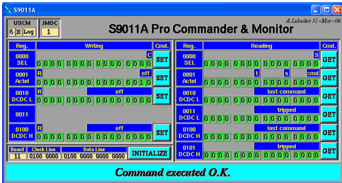
Figure C.1: This screenshot shows the S9011AU commanding software that was used during the development of the firmware and will be used during the various tests of the S9011AU. It will also serve as a basis for the final software, which will be used during the flight. [Software by Alexei Lebedev]
