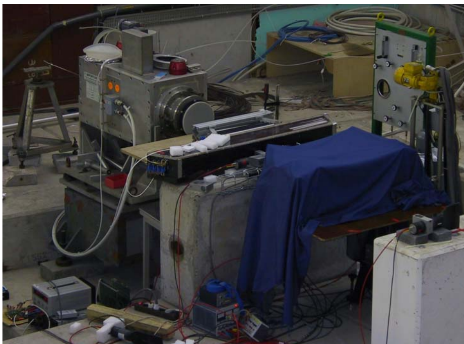
Figure 2.52: The setup used during the beam test at the PS facility at CERN in October 2002. The beam entered from the right side of the picture and then passed through a set of trigger scintillators, prototype scintillators for the anti-counters of AMS02, hidden beneath the cloth, through the two TRD jigs and finally through a Multi-Wire Proportional Chamber (MWPC), which was not used during our measurements.
