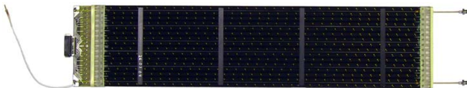
Figure 1.8: A strawtube module of the AMS02 TRD. Each of the 328 modules of the TRD consists of 16 proportional gas tubes constantly flushed with a Xenon- \text{CO}_2 mixture (80:20). The length of the modules ranges from 80 \text{ cm} to 200 \text{ cm} , depending on their position in the octagon.
