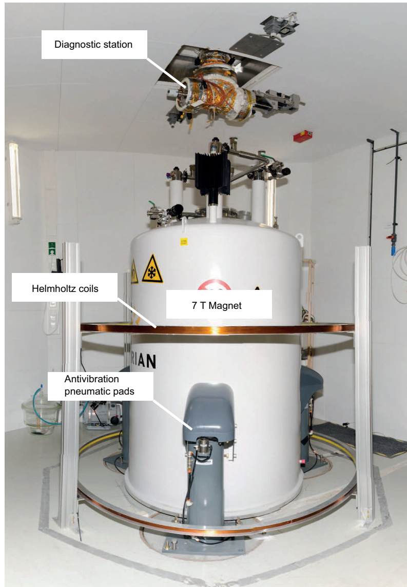
Figure 6.6: Photograph of the PENTATRAP magnet. On the top, a part of the beamline towards the ion source is shown with the beam diagnostic station attached. The magnet is placed on antivibration pneumatic pads in the center of the Helmholtz coils, which are used to reduce environmental magnetic fluctuations.
