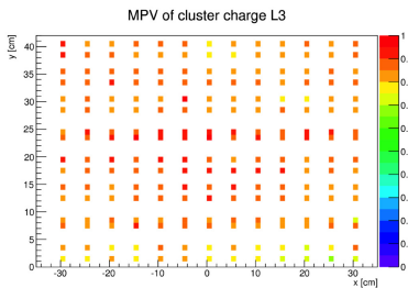
Figure 6: 2D distribution of the mean cluster charge normalized to the maximum value
