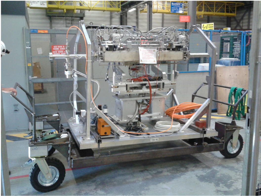
Figure 6.1: The collimator tank mounted on the fully assembled table to be lowered to the HiRadMat experimental area.
