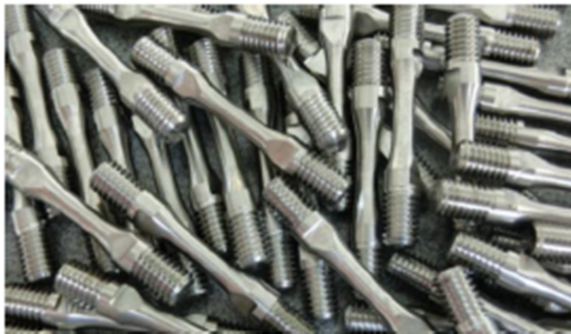
Figure 5.17: Specimens of INERMET® 180 used for the structural characterisation tests: schematic diagram of the standard dumbbell (dog-bone) shaped specimen used for the tensile tests ( \phi = 3 mm, L = 5 mm) (top), and 60 samples of INERMET® 180 used for the experimental test campaign (bottom).
