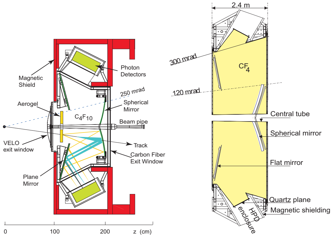
Figure 2.24: Left: schematic layout from a side view of the RICH 1 detector. The Cherenkov light as emitted by a charged track traversing the Aerogel tiles and the C_4F_{10} radiator is also drawn. Right: Schematic layout from a top view of the RICH2 detector.
