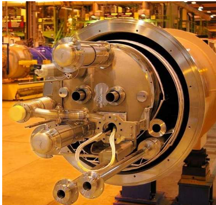
Figure 3.2: Profile of one of the 15m long cryodipoles of the LHC [25]
