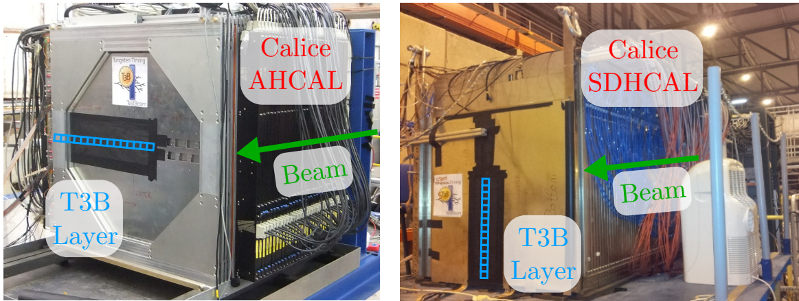
Figure 4.13: Pictures of the test beam setup of the T3B experiment together with the CALICE tungsten AHCAL (left) and the CALICE steel SDHCAL (right). The position of the scintillator cells of T3B is indicated by a blue strip.
