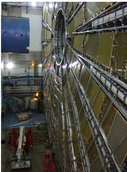
Figure 3.7: End caps of the muon spectrometer [40]
