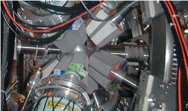
Figure 3.9: One hemisphere of the GASP detector system used for the ^{170}\text{Er} experiment.
