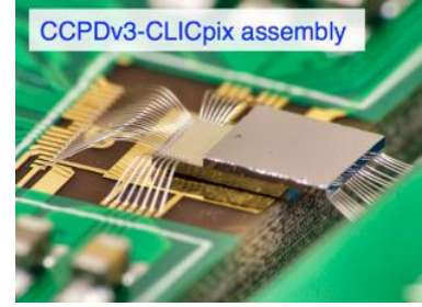
Figure 5: Hybrid glue assembly of a CLICpix prototype chip with a CCPDv3 active sensor on top
