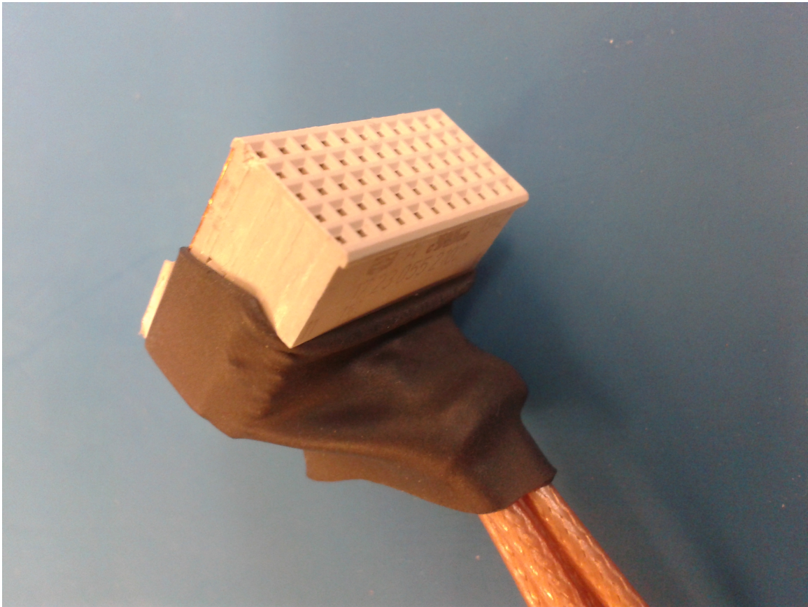
Figure 7.3: A picture of the patch cable for the LDTB.
