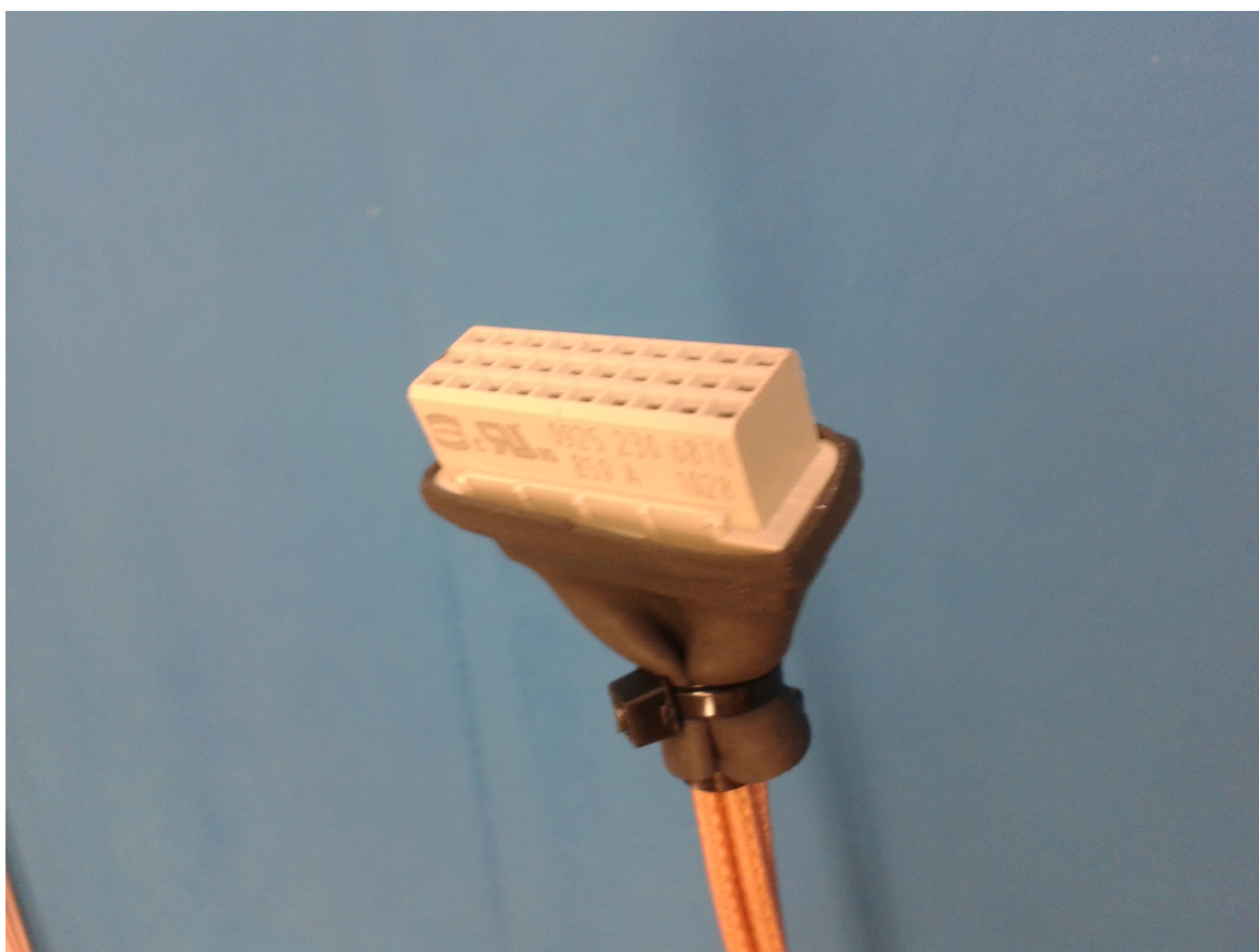
Figure 7.4: A picture of the patch cable for the FEB and TDB.
