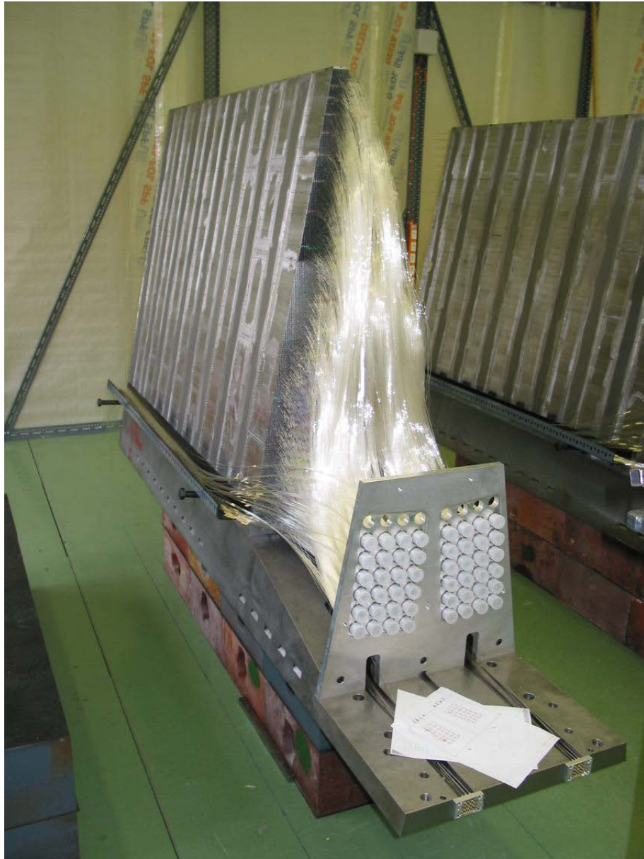
Figure 1.4: Photograph of HF wedge.
