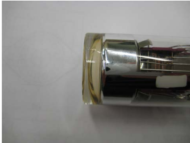
Figure 2.10: A picture of the HF PMT glass section. The glass shape is plano-convex and the thickness in the center (1 mm) increases towards the edges (6.1 mm). Interaction of relativistic particles with glass create Cerenkov photons.
