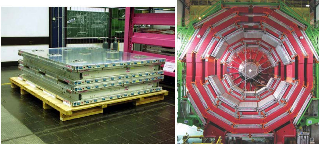
Figure 3-32. Left: photo of Drift Tube (DT) chambers awaiting shipment to CERN. Right: as installed in the barrel region (Copyright CERN).
