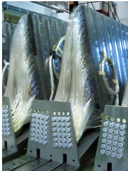
Figure 3-29. Photograph of wedges of the Forward Calorimeter (HF) awaiting installation (Copyright CERN [43]).
