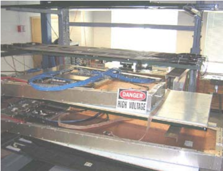
Figure 3-34. This cosmic test stand was constructed at the University of Florida in support of CSC commissioning.
