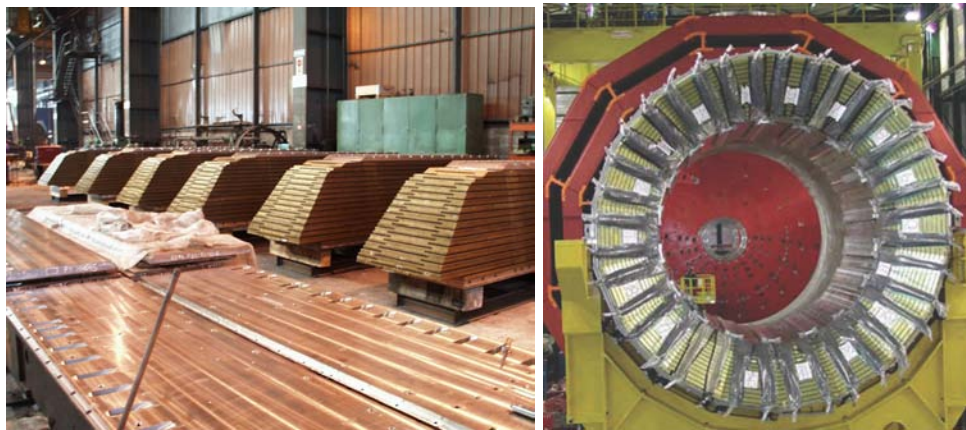
Figure 3-27. Left: a series of HB wedges awaiting assembly. Right: merged together to form the HB sub-detector (Copyright CERN).
