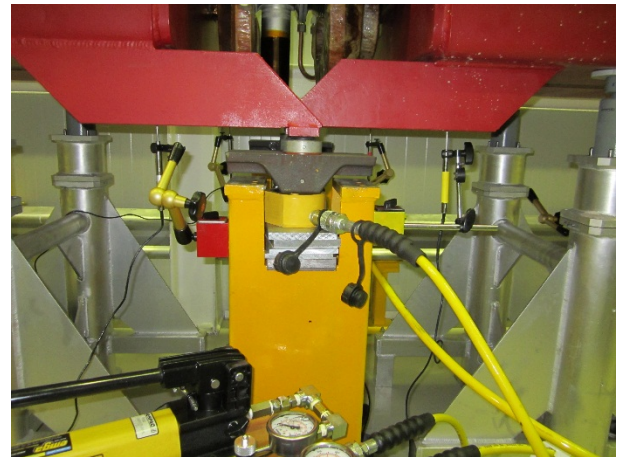
Figure 4: Dipole interconnect handling equipment
