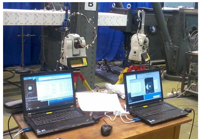
Figure 3: Two QDaedalus systems on robotic total stations Leica TDA5005.
