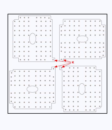
cross shield: 4 EC provide full shield for 4 MaPMT
