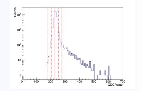
Spectrum of QDC values in small magnetic field (left) and high magnetic field (right), for the MaPMT R11265 operated at 1 kV. The red solid line indicates the pedestal mean, the dotted lines show  $Q_0 \pm 5\sigma$  and  $Q_0 \pm 10\sigma$ .
