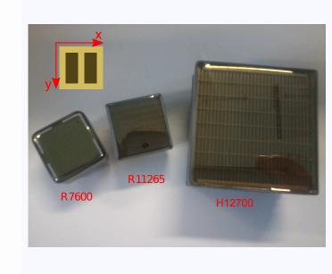
Two candidates tested: R7600 and R11265, 1" Hamamatsu 64-channel ( $8 \times 8$  pixels) Multi-anode Photomultiplier. R11265 preferred: bigger active area (77% vs 50%) and better separation of the single photo-electron signal from noise.
