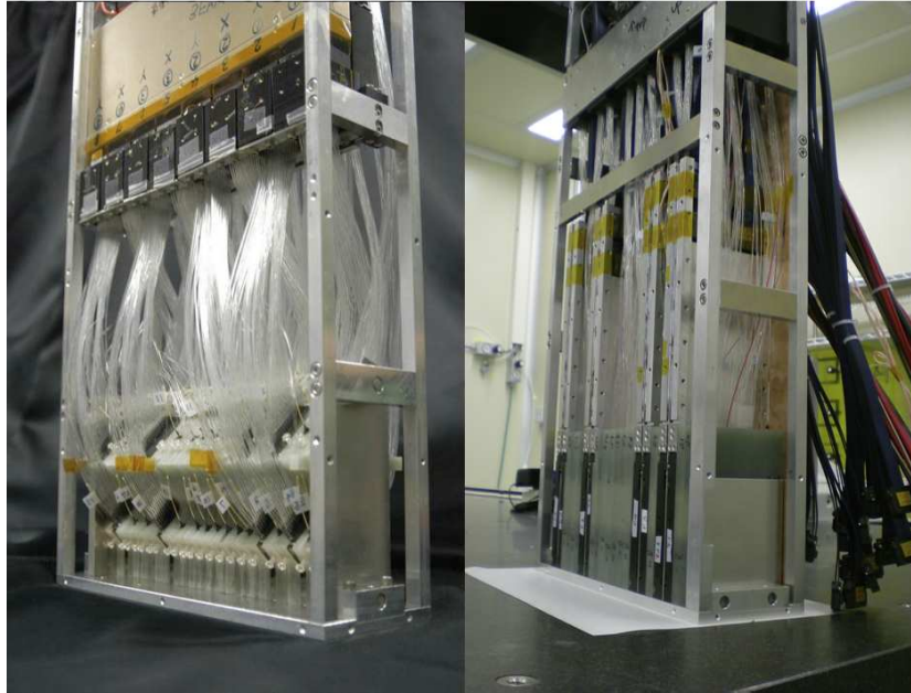
Figure 2.7: Pictures of the LHCf detectors. Left panel shows the Arm1 detector, and right shows the Arm2 detector.
