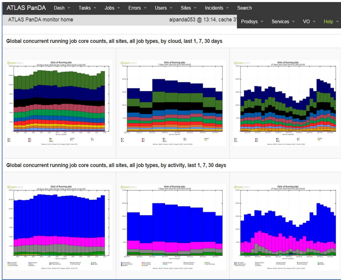
Figure 4. The front page of new monitoring shows history of the number of CPU cores used by concurrently running jobs per regional federation (top row) and per activity (bottom row) for 1, 7 and 30 days, respectively. There are also hyper-links to various monitor pages, such as task-oriented views and job-oriented views.
