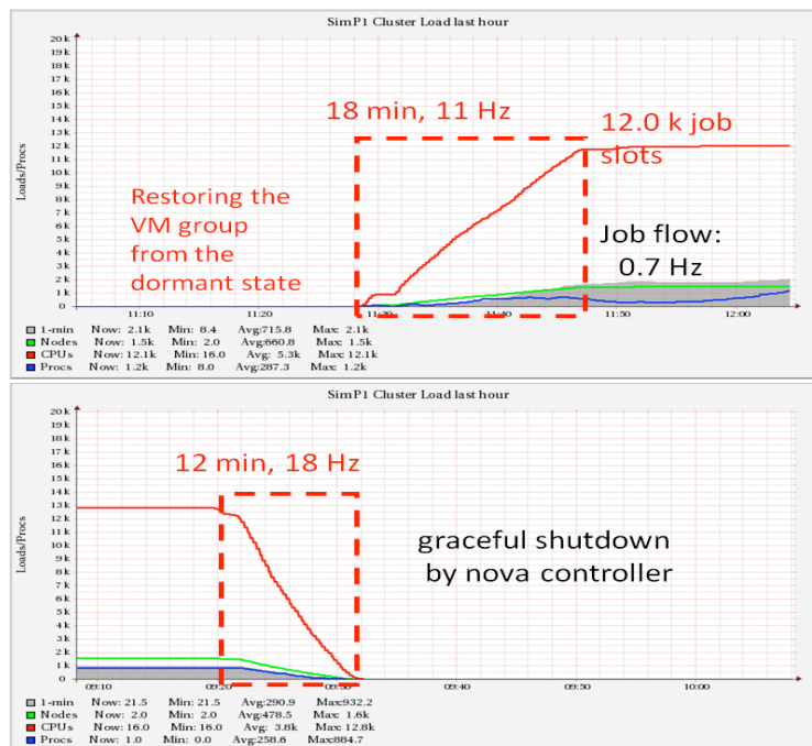
Figure 4. Measurement of VM startup and graceful shutdown times for Sim@P1.
