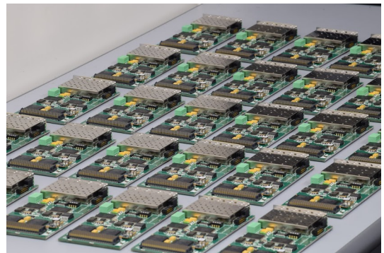
Fig. 3. Mass production of 80 FTK_IMs are done. Quality control test will be performed, and they will be delivered to CERN after completing the quality control test.
