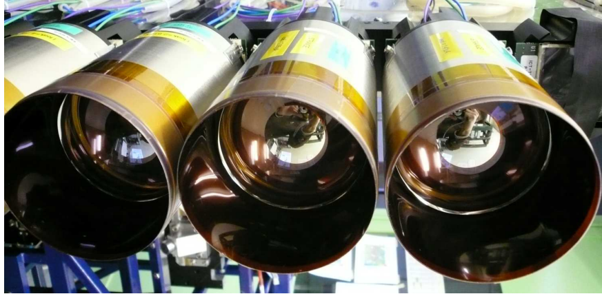
Figure 3.3: HPDs with Mu-metal shieldings.
