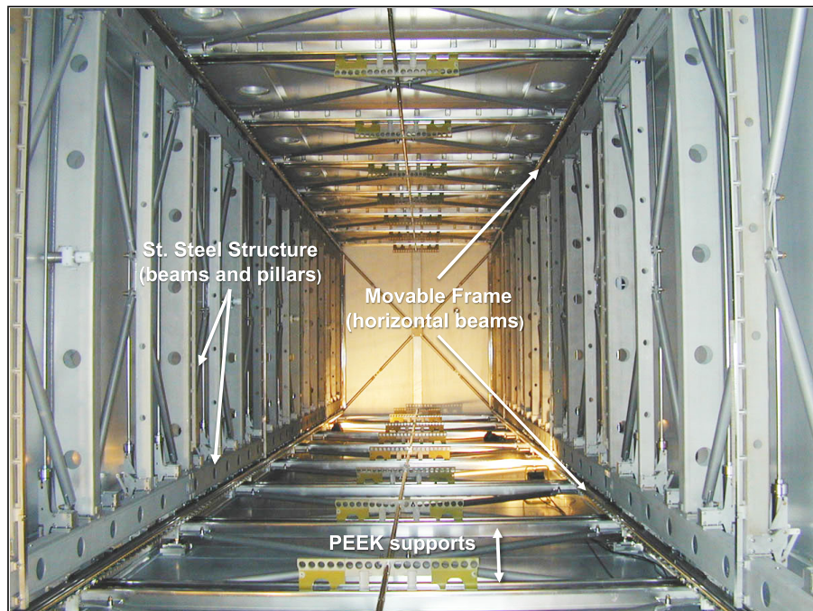
FIG. 67: The internal sustaining structure of a T600 module.
