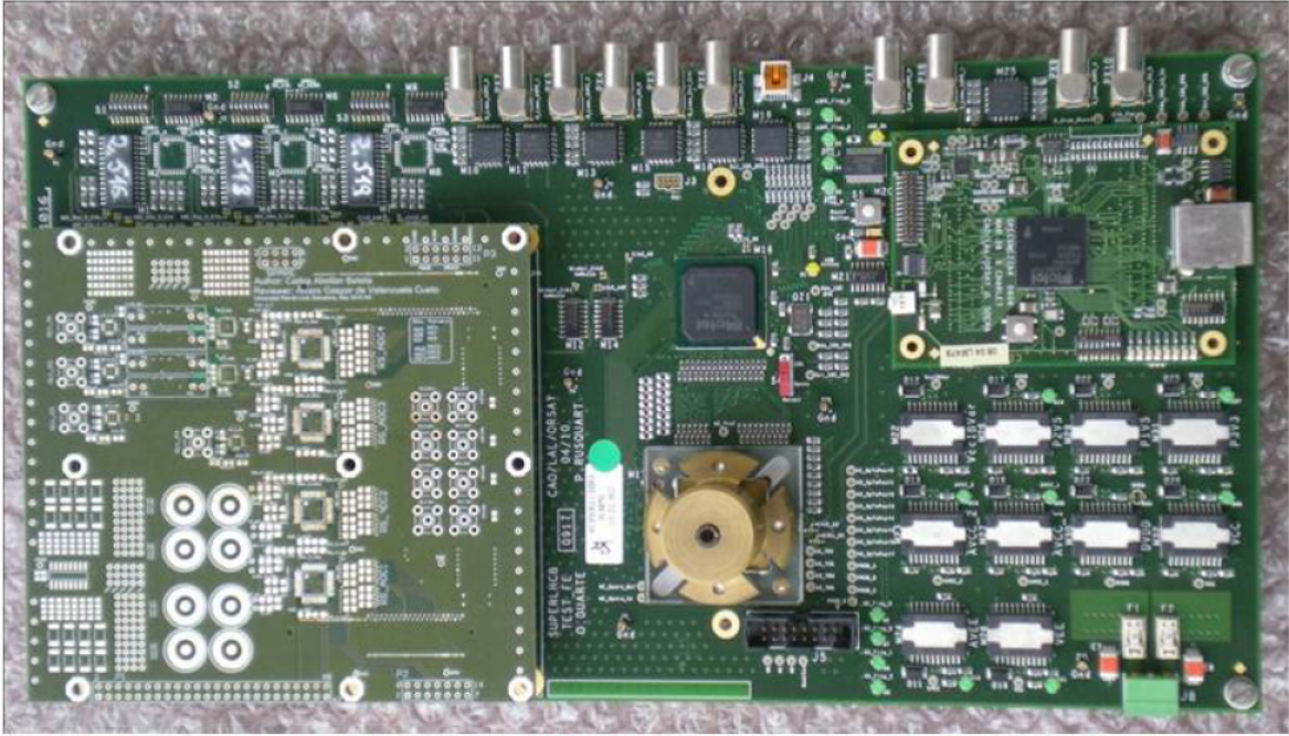
Figure 7.1: Picture of the prototype of the Front-End board. The analogue mezzanine is visible on the left. The two FPGAs are in the central part of the board, one is black and other is under the copper socket.
