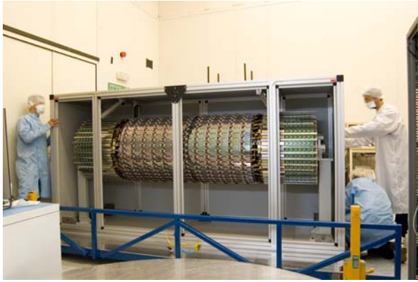
Figure 5.6: SCT barrel 4 being prepared for shipping to CERN.
