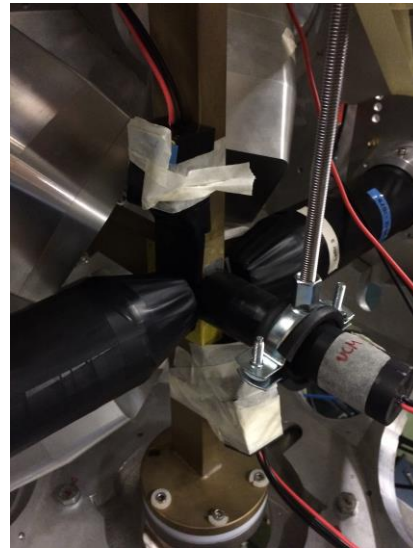
Figure 1: Left: Picture of the IDS set-up showing the tape station, surrounded by the Clover HPGe detectors. Right: Close view of the fast-timing ancillary detector set-up.
