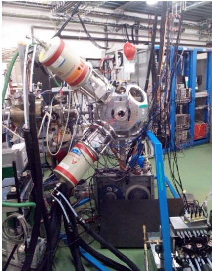
Figure 1: Left: Picture of the IDS set-up showing the tape station, surrounded by the Clover HPGe detectors. Right: Close view of the fast-timing ancillary detector set-up.
