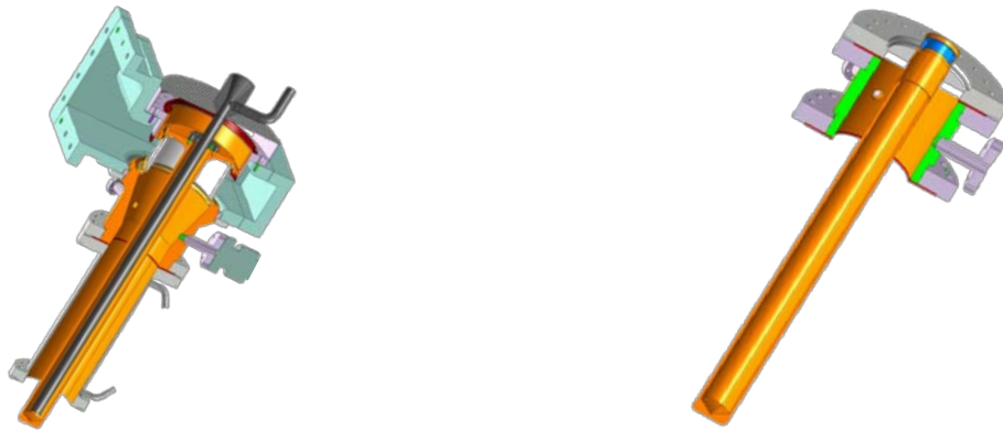
Figure 34: SPL power couplers: Cylindrical window type (left) and flat window type (right)
