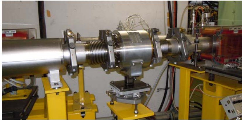
Figure 14: New Inductive BPM in the GPS Isolde line.
