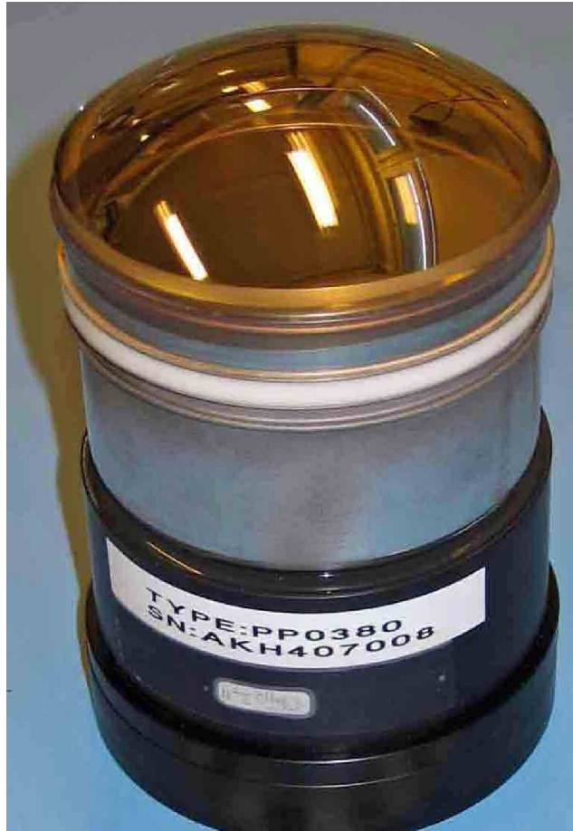
Figure 3.10: Photograph of one of the HPDs used inside the RICH detector. Reproduced from Ref [28].
