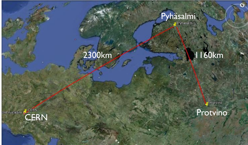
Figure 1. View of the dual beamline configuration: CERN to Pyhäsalmi (2300 km) and Protvino to Pyhäsalmi (1160 km).
