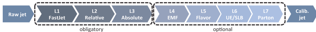
Figure 4.5.: The factorized jet energy correction approach: Each level corrects for a different jet- p_T bias. The first three correction levels are obligatory, while the latter correct for analysis specific effects.
