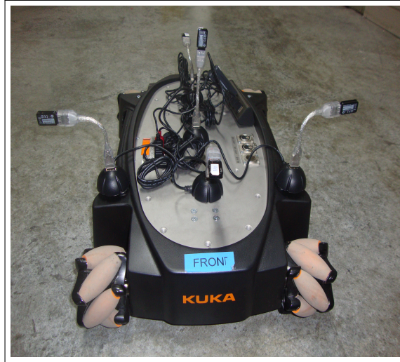
Figure 4.5: youBot mobile robot used in the tests. Many wireless receivers are mounted on the youBot in different orientations.
