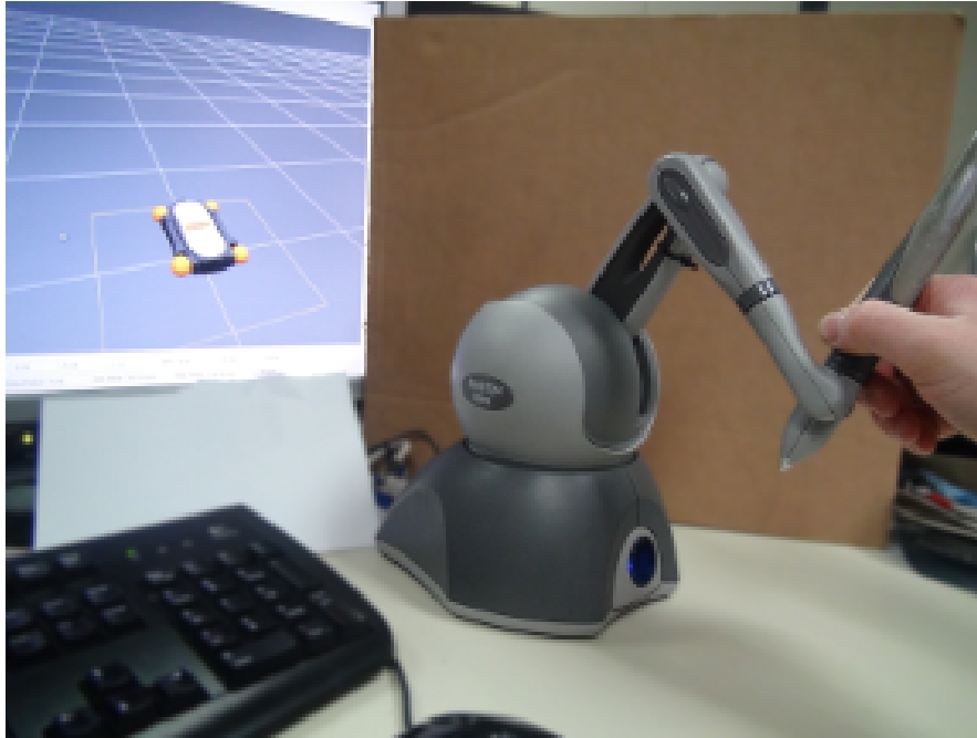
Figure 5.8: PHANTOM OMNI slave controller is used to control the youBot simulated using ROS.
