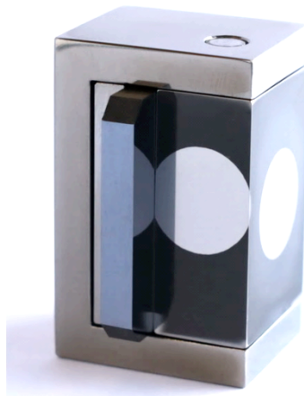
Figure 6 : quasi-mosaic crystal in its bending support, produced by PNPI, Gatchina. The silver spots are the polished regions of the support orthogonal to each other for alignment.
