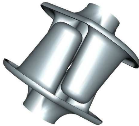
(c) Interleaved rods of the cavity with gap between rods for cutting.
