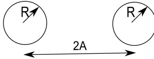
Figure 2.16: Two rod transmission line, each rod has radius R and the mid points of the rods are separated by a distance of 2A
