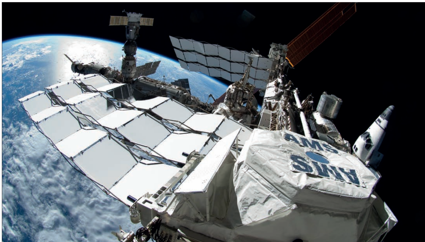
Fig. 1. The CO 2 cooling system (single panel, centre) for the AMS on board the International Space Station. (Image credit: NASA.)
