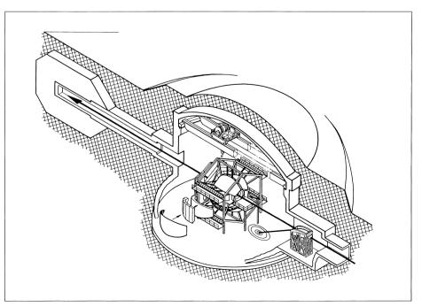
superconducting coils arranged symmetrically around the beam beamline will generate CLAS' magnetic field.
