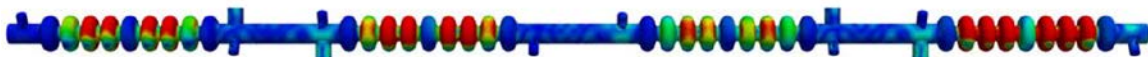
Fig. 12 Sample of ACE3P output (displayed in Paraview) showing the 3D magnitude of the electric field distributions of the trapped mode at 9.061 GHz from the 5th dipole band.
