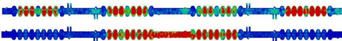
Fig. 17 ACE3P magnitude electric field distributions from the 5th dipole band: 9.061 (top, trapped mode) and 9.062 (bottom, inter-cavity mode).
