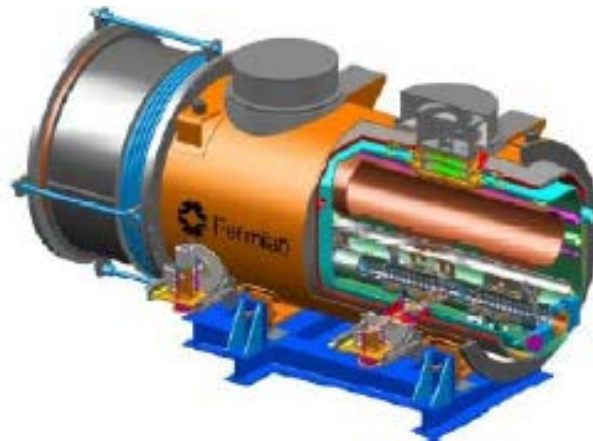
Fig. 3 Schematic of FNAL cryo-module consisting of four 3.9 GHz cavities (Diagram courtesy FNAL).
